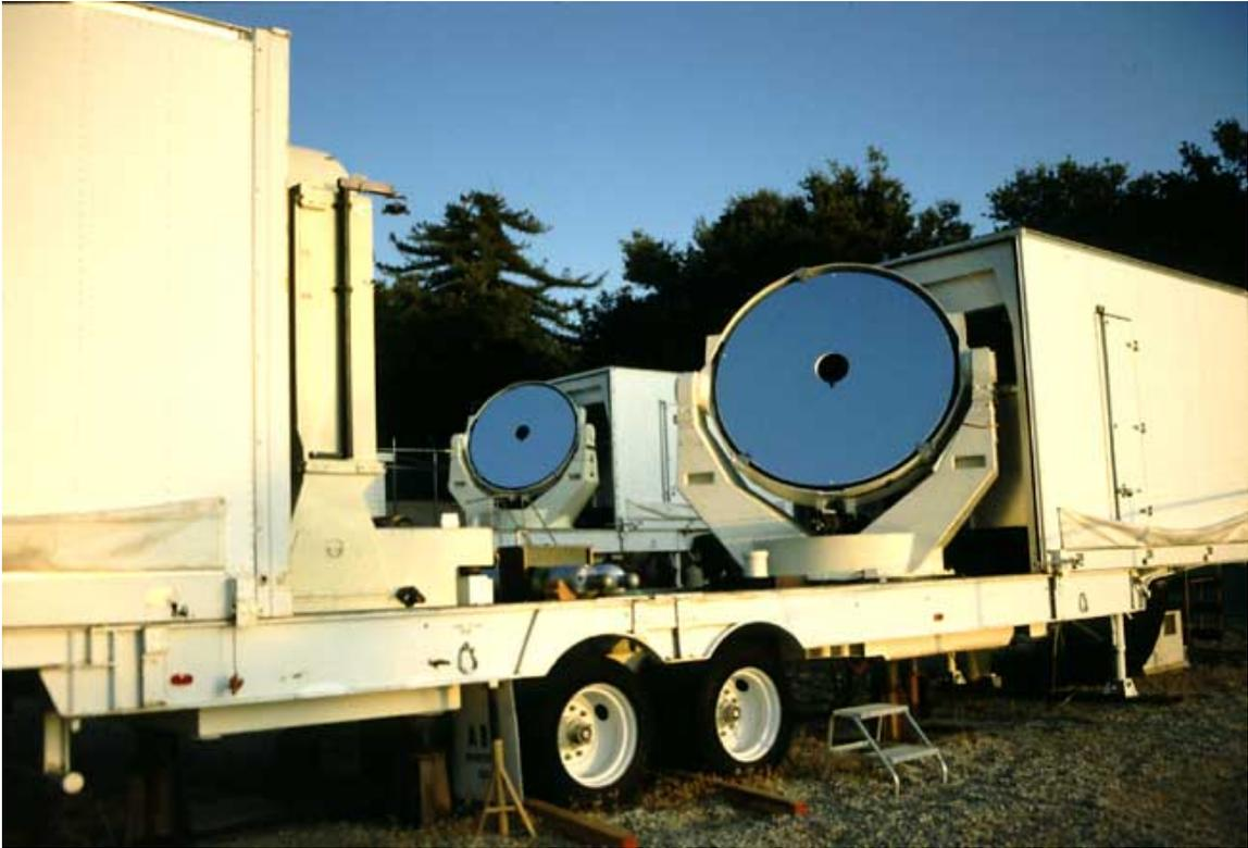
**Figure 1:** U.C. Berkeley Infrared Spatial Interferometer is shown on its initial 4 m baseline at Mt. Wilson in Southern California. Visible are the two telescopes, each of 65” aperture, which are mounted in modified semi-trailers. Each telescope consists of a flat mirror that tracks the source and a parabolic mirror that is fixed, the latter barely visible on the left of the trailer in the foreground. The parabolic mirror focuses the light through a hole in the flat mirror.
